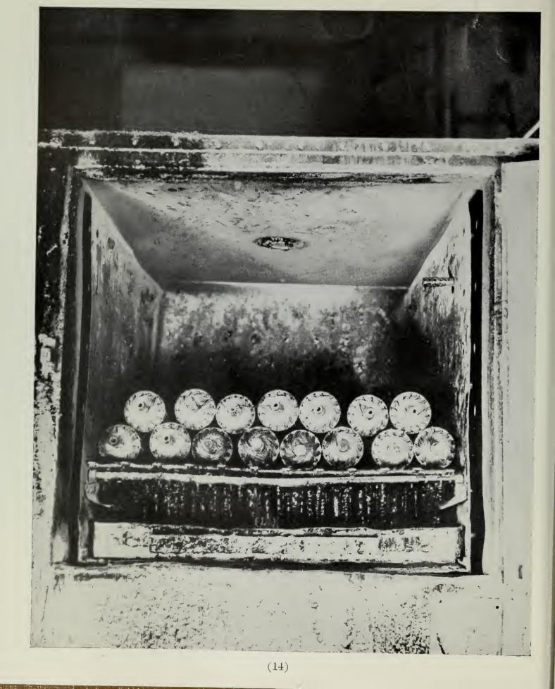
The armatures are placed in an electric oven, as shown above, and baked overnight at a temperature of about two hundred and fifty degrees.
